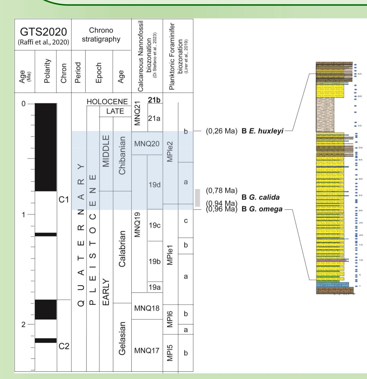
The age of Tol-1 has been estimated using calcareous nannofossils. The bottom occurrences of *Gephyrocapsa omega* and of *Emiliania huxleyi* constrain its age between 0.96 Ma and, at least, 0.26 Ma (according to the new Mediterranean calcareous nannofossil zonation proposed by DI STEFANO *et al.*, 2023), thus spanning from late Calabrian to late Chibanian.
